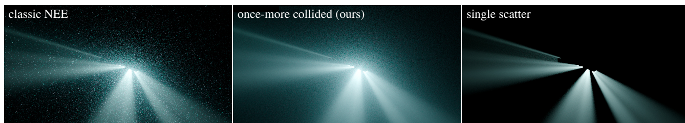
Figure 16: Once-more scattered next event estimation evaluated towards a light source, i.e. in path tracing from the camera. The images show the importance of the extra scattering vertex on top of single scattering only (right), and also demonstrate how our technique can robustly reduce the noise in this setting. All images are 1024 samples per pixel.
